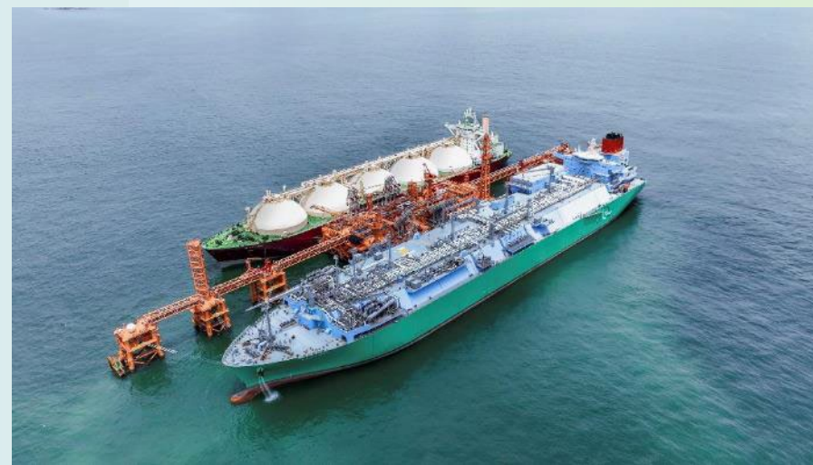
The Floating Storage and Regasification Unit (FSRU), LNG carrier and offshore LNG terminal in Hong Kong
