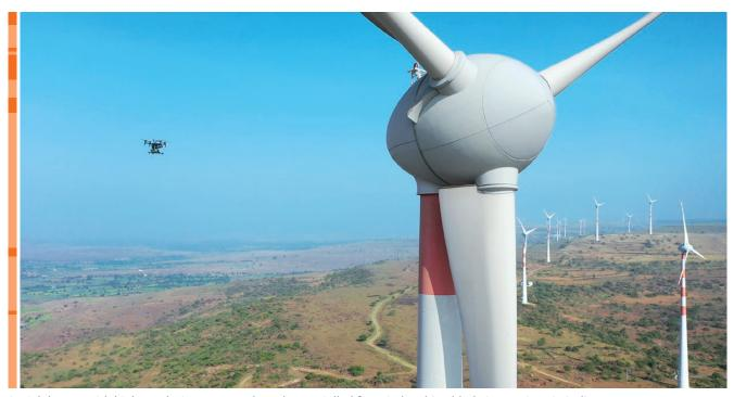
Aerial drones with high resolution cameras have been trialled for wind turbine blade inspections in India.
