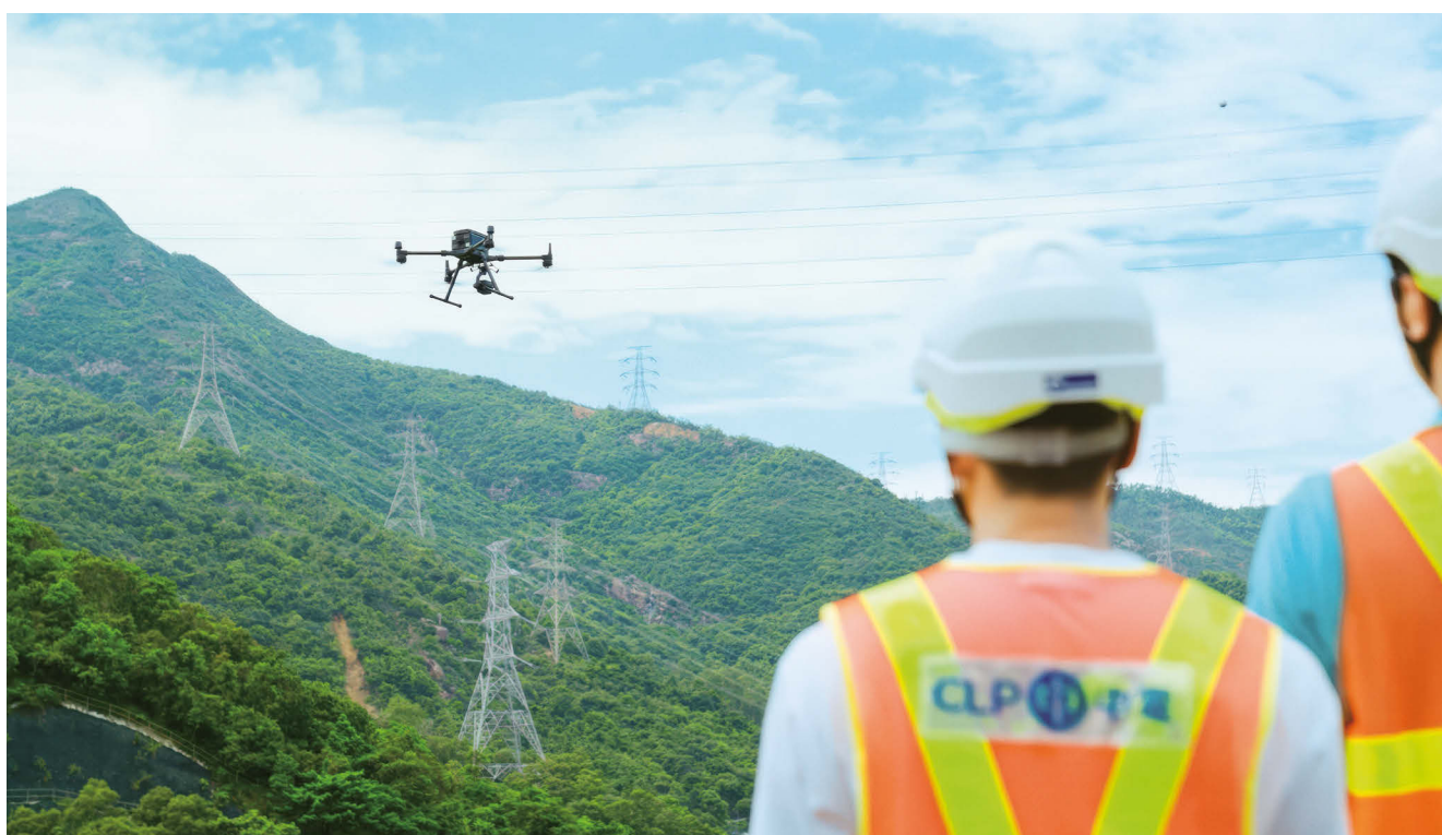
CLP Power adopts advanced technologies such as Beyond Visual Line of Sight drone operations to enhance the efficiency of power facility inspections.
