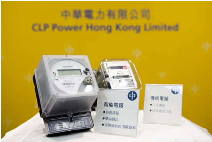
(Photo 2) Smart meter (left) and traditional meter (right)
