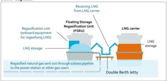
The operations of an offshore LNG terminal using floating storage regasification technology.
