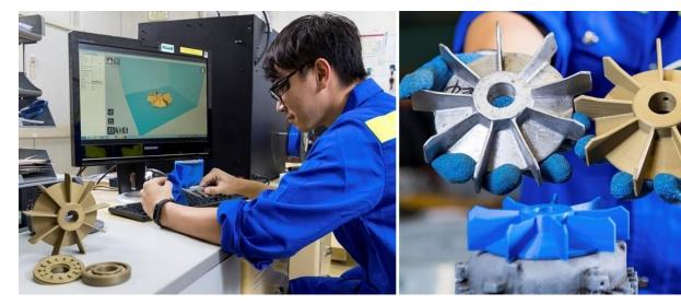
GBG engineers first experimented with 3D printing in December 2016. Since then, they have applied it in making parts for cooling fans, switches and insulators.
