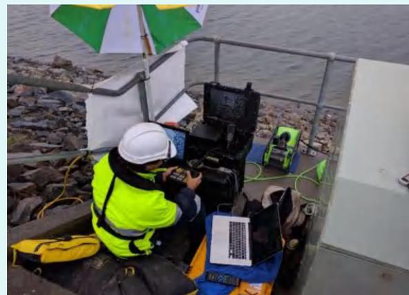
ROVs are used for inspecting the cooling water inlet tower in the Mount Piper thermal plant in Australia.
