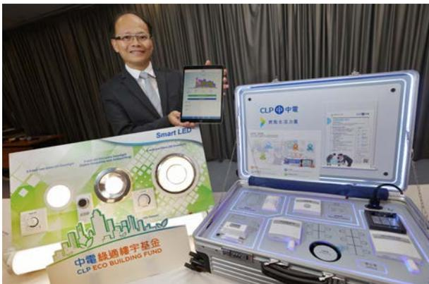
Under the upgraded CLP Eco Building Fund, the implementation of smart technology and devices are eligible for funding. CLP Power Acting Director of Corporate Customer Experience Dr Anthony Lo shows examples of smart sensors, which can remotely monitor, pre-set, and control lighting and air conditioning systems in buildings, and help manage energy more effectively.
